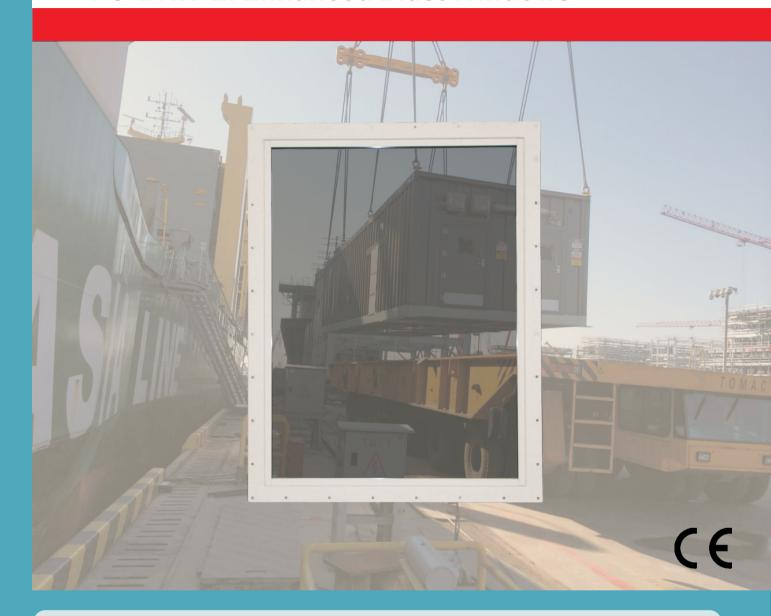
FC-BRW-EI enhanced blast windows are designed to provide blast protection up to 2 bar reflected by long duration or up to 5 bar reflected by 5ms. FC-BRW-EI enhanced blast windows can remain fully functional after one or multiple blast hits thanks to design that all the components, including frame and laminated glass layers, work in elastic range under the blast grade mentioned.
